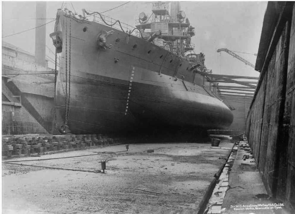
HMS Glatton's partially water-filled anti-torpedo bulges
