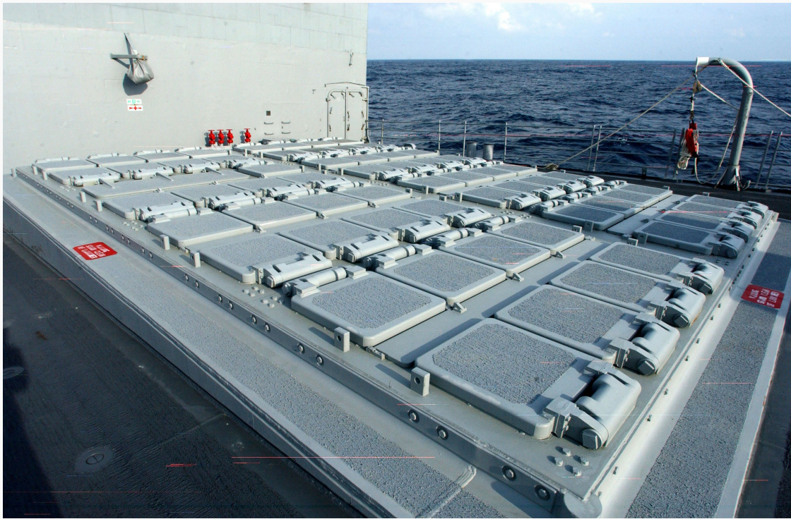
A topside view of the forward MK-41 Vertical Launching System (VLS) aboard the guided missile cruiser USS San Jacinto
